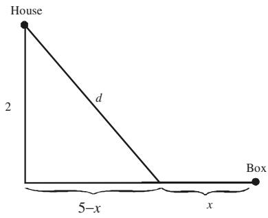
$$\begin{aligned}d &= \sqrt{(5-x)^2 + 2^2} \\&= \sqrt{25-10x+x^2+4} = \sqrt{x^2-10x+29}\end{aligned}$$
