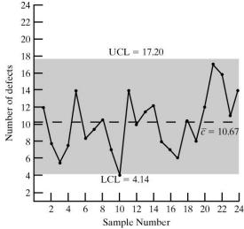
The process does not appear to be out of control, but sample 21 is close to the UCL and the process should be investigated.
