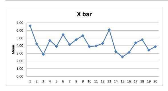
The process appears to be in control, with sample 1 seeming to be an aberration, however, the process should still be checked.
