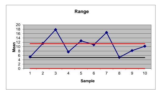
The process clearly seems to be out of control. There are three of the sample points above the UCL, and all other sample values are above the centre line for  $\overline{R}$ , indicating nonrandom variations.
