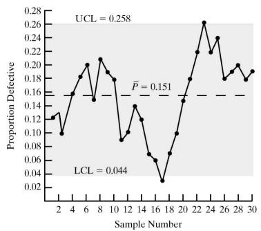
The process does not seem to be out of control, although the decreasing number of defects from sample 8 to sample 17 should probably be investigated to see why the steady improvement occurred; likewise, the steadily increasing number of defects from sample 17 to sample 25 should probably be investigated to see why the quality deteriorated.
