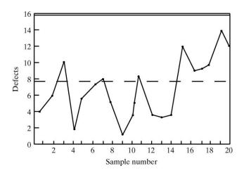
The process appears to be in control however the process may be moving toward an out-of-control situation.
