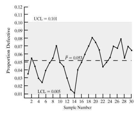
The process does not seem to be out of control.
