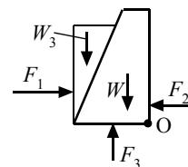
$$\begin{aligned}\Sigma M_O &= 706.32 \times 4 + 264.9 \times 4.5 + 397.3 \times 6 - 546.7 \times 0.9 - 1093.4 \times 4.2 \\ &\quad - 412.02 \times 6.27 - 44.14 \times 1 \\ &= -851.2 \text{ kN-m} < 0 \text{ and hence the dam won't tip.}\end{aligned}$$
