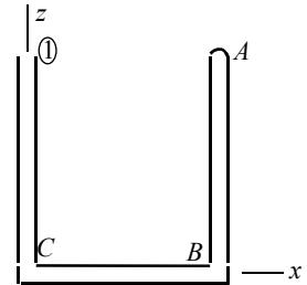
$$\text{b) } p_A = -1000 \times a_x = 10 \text{ m/s}^2 (0.9 - 0) = -9000 \text{ Pa} = \underline{-9 \text{ kPa}}$$
