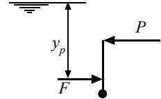
$$y_p = \bar{y} + \frac{\bar{I}}{\bar{y}A} = 3.3 + \frac{1.8 \times 3^3 / 12}{3.3 \times 1.8 \times 3} = 3.53 \text{ m.}$$
