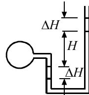
2.40  $p + 9810 \times 0.05 + 1.59 \times 9810 \times 0.07 - 0.8 \times 9810 \times 0.1 = 13.6 \times 9810 \times 0.05.$
