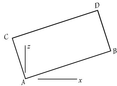
$$\text{b) } p_D = 0. \quad p_C = -1000 \times 17.32 (-0.5 - 1.232) - 1000 \times 19.81 (0.866 - 1.866) = 49\,810 \text{ Pa.}$$
