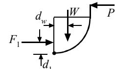
Note: This calculation is simpler than that of Example 2.7. Actually, We could have moved the horizontal force  $F_H$  and a vertical force  $F_V$  (equal to  $W$ ) simultaneously to the center of the circle and then  $2.5P = 2F_H = 2F_1$ . This was outlined at the end of Example 2.7.
