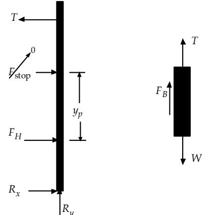
$$F_H = \gamma \bar{h} A = (9.81 \text{ kN/m}^3)(1.5 \text{ m} \times 6 \text{ m}^2) = 88.29 \text{ kN}$$
