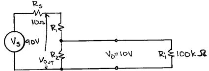
For a loading error of 0.1%, the voltage drop across  $R_s$  should be  $90\times0.001 = 0.09$  V. The current through  $R_s$  is then:
