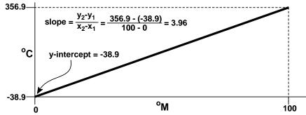
Therefore, the equation for the line is y = 3.96x - 38.9 The algebraic relationship between the two temperature scales is
