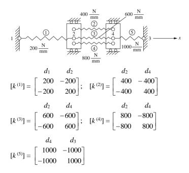
Assembling global [K] using direct stiffness method
