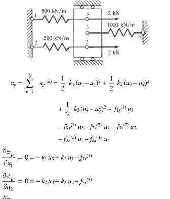
$$\frac{\partial u_p}{\partial u_3} = 0 = k_1 u_3 + k_2 u_3 - k_2 u_2 - k_3 u_4 + k_3 u_3 - f_{3x}^{(2)} - f_{3x}^{(3)} - f_{3x}^{(1)} - k_1 u_1$$
