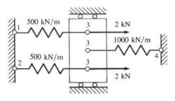
$$[k^{(1)}] = \begin{bmatrix} 500 & -500 \\ -500 & 500 \end{bmatrix}; [k^{(2)}] = \begin{bmatrix} 500 & -500 \\ -500 & 500 \end{bmatrix}; [k^{(3)}] = \begin{bmatrix} 1000 & -1000 \\ -1000 & 1000 \end{bmatrix}$$
