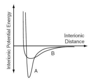
The well of titanium, represented by A, is deeper (higher melting point), has a larger radius of curvature (stiffer), and is more symmetric (smaller thermal expansion coefficient) than the well of aluminum, represented by B.
