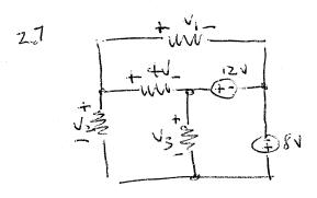
$$V_1 - 12 - 4 = 0 \implies V_1 = 16V$$
