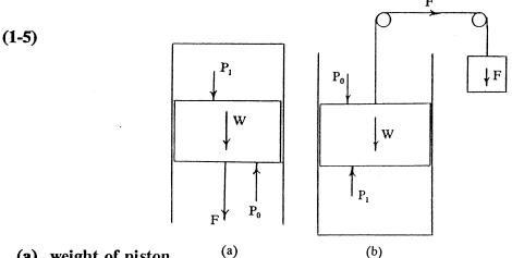
(a) weight of piston (a) (b)  $W = mg/g_c = [(2700 \text{ kg})(9.81 \text{ m/sec}^2)]/[(1 \text{ kg-m/N-sec}^2)(1000 \text{ N/kN})] = 26.487 \text{ kN}$
