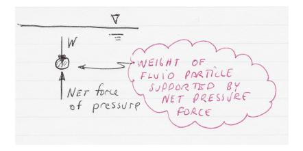
• Engineers establish hydrostatic conditions by analyzing the forces acting in the z-direction.
