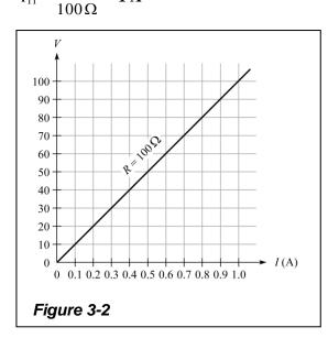
The graph is a straight line as shown in Figure 3-2. This indicates a *linear* relationship between *I* and *V*.
