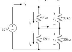
$$6 \text{ k}\Omega \| 30 \text{ k}\Omega = 5 \text{ k}\Omega$$
