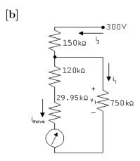
$$v_1 = (0.96 \text{ m})(150 \text{ k}) = 144 \text{ V}$$
