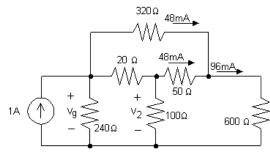
$$v_2 = (50)(0.048) + (600)(0.096) = 60 \text{ V}$$
