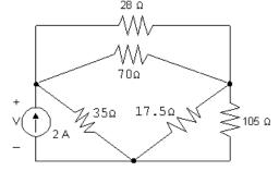
From this circuit we see that the  $70\,\Omega$  resistor is parallel to the  $28\,\Omega$  resistor:
