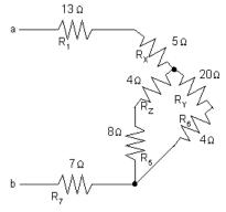
Now calculate the equivalent resistance  $R_{ab}$  by making series and parallel combinations of the resistors:
