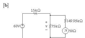
The meter resistance is a series combination of resistances:
