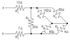
Make series and parallel combinations of the resistors to find the equivalent resistance  $R_{ab}$ :
