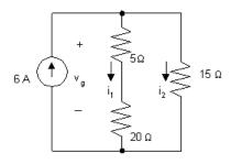
$$i_1 = \frac{(6)(15)}{(40)} = 2.25 \text{ A}; \quad v_x = 20i_1 = 45 \text{ V}$$
