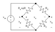
$$v_{\rm a} = \frac{v_{\rm in}R_4}{R_0 + R_4 + \Delta R}$$
