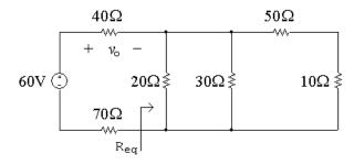
[a] First we need to determine the equivalent resistance to the right of the  $40\,\Omega$  and  $70\,\Omega$  resistors:
