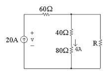
[a] We will write a current division equation for the current throught the  $80\Omega$  resistor and use this equation to solve for R:
