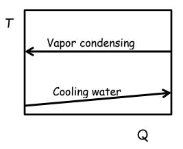
b. Distillation reboiler using condensing steam as the heating media
