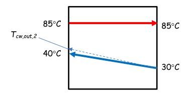
a. If the limiting resistance is on the cooling water side, what is the maximum scale-down possible based on the condenser conditions without incurring a financial penalty? What is the new outlet temperature of cooling water? By what factor must the cooling water flow change?
