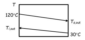
$$\Delta T_{lm} = \frac{(120 - T_{i,out}) - (T_{s,out} - 30)}{\ln \frac{(120 - T_{i,out})}{(T_{s,out} - 30)}}$$
