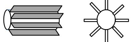
For each fin,  $\delta$  = 0.00075m, *L*= 0.015 m, *L*<sub>tube</sub> = 3 m, From Equation 2.79m *L<sub>c</sub>* = *L*+ $\delta$ /2=0.015+0.00075/2= 0.01538m From Equation 2.69,
