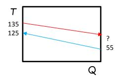
Energy balance gives  $(135 - T_{1,out}) = \frac{(6.4925)}{(7.1400)}(125 - 55) \Rightarrow T_{1,out} = 71.35^{\circ} \text{C}$
